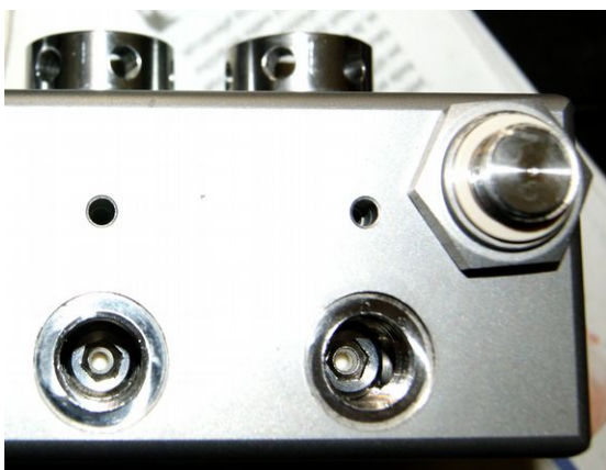
Fig. 7: Hexagonal caps and valves inside head, back side tightening screws
