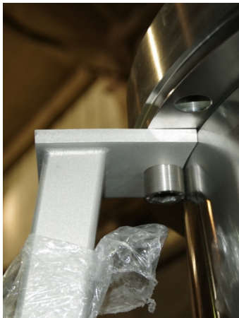
Fig. 6: Leg on the upper flange
