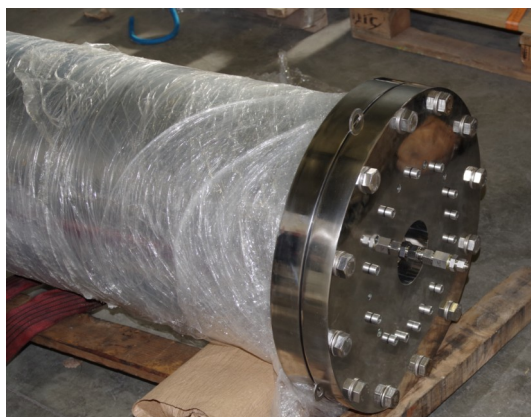
Fig. 2: Column tube with bottom flange
