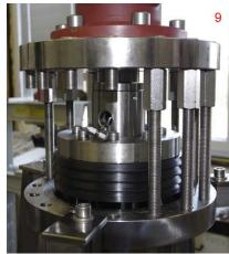
leg support plate made of 5 mm thick steel connected to rods by 6 sleeves On one leg are connected panel for flow reversation and UV detector remote cell (Fig 12, 13). Both panels are connected to the leg by bolts M6.
