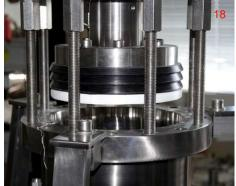
Hydraulic piston is moved down carefully to reach the smallest gap between CP 11 and CP 2. Three bolts on CP 2 hate to be released during this procedure and they are slightly tightned when CP 1 is inside the grove on upper part of CP 2. The whole is moved a bit up and metal sheet is removed.
