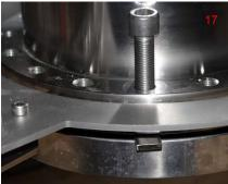
must be pull on the column tube (Fig. 1 on the front page). When rods are installed and the plate laying on them, it is connected to rods by delivered 6 sleeves (each 2 on 1 rod).
