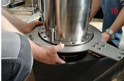
and than with 20 I of destilled water. Than there is no organic solvent inside the column. Proper vessel with volume 20 I or more is installed under the column bottom flange. The column output is closed and bottom flange bolts are released and the whole flange is pressed out of the column (two men must keep in hands (Fig. 19) by the pressure of water which is pumped inside the column by mobile phase pump.
