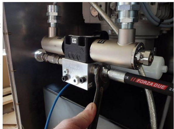
Fig. 18: Hydraulic hoses connection
