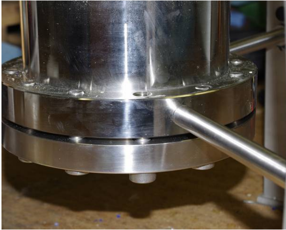
Fig. 10 Bottom piston unit assembled to a bottom tube flange and side leg rod installation
