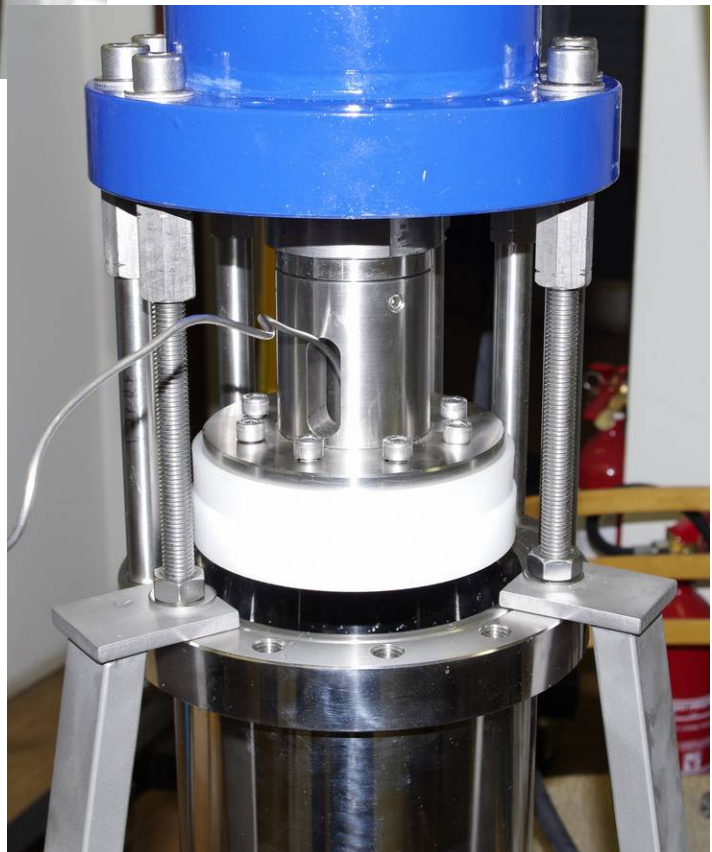
Fig. 11 Upper piston unit inserted into hydraulic piston supporting rods
