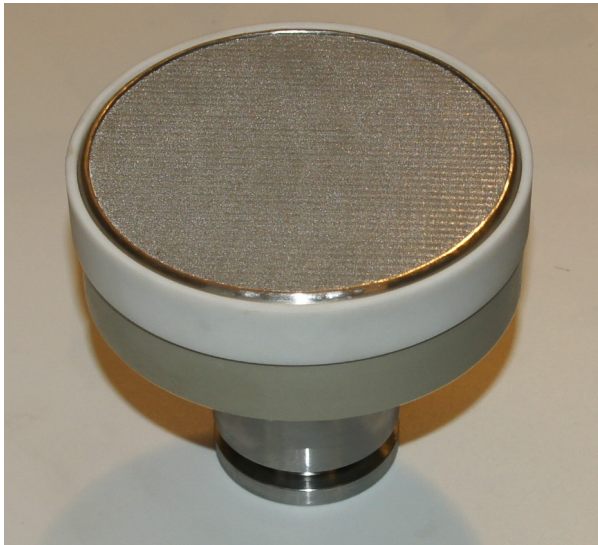
Fig. 7 Upper piston with seal rings and support
