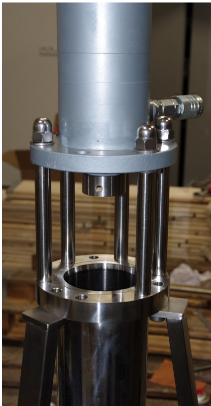
Fig. 9 Column with distance tubes and hydraulic cylinder
