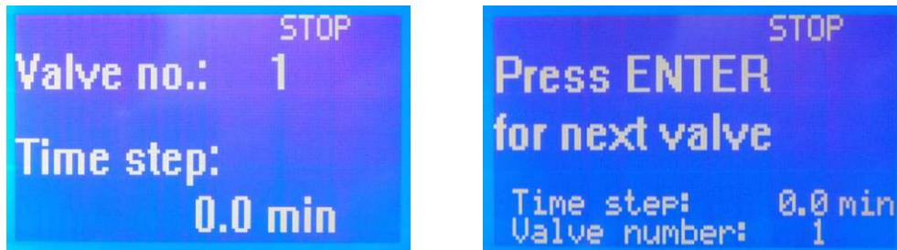
Press the F1 button again to check the set residence times on the valve, then "Settings Time 4". The time for the valve 5 is no longer set since the collector ends there when it is not stopped on the previous valve. If we do not want to use all the valves, the last used time is set = 0.0 min.
