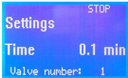
After checking the set values, use the F2 button to return to the default item and start the START / STOP button. When pressed, the state in the upper right corner will change to RUN and the collector will begin counting the residence time on the individual valves.
