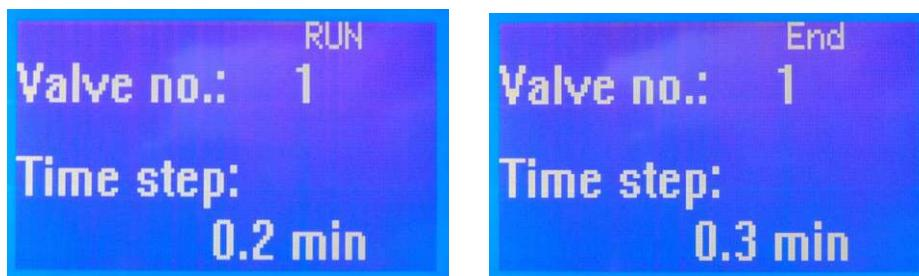
Press the START / STOP button to stop the collector on the current valve ("End" appears in the top right corner). Pressing the START / STOP button again returns the collector to the starting valve 1.
