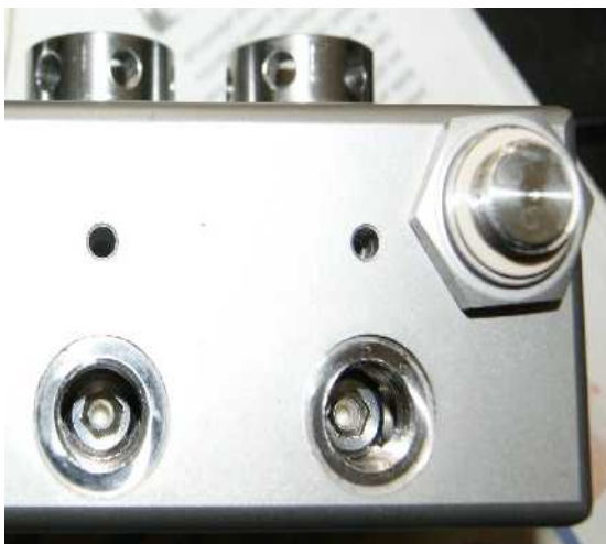
Fig. 7: Hexagonal caps and valves inside head, back side tightening screws
