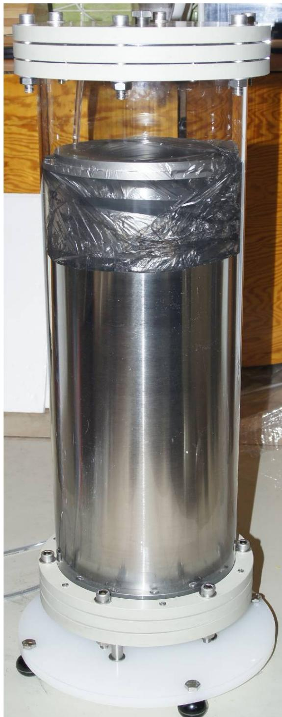
Fig. 10 Thermostating jacket fully assembled
