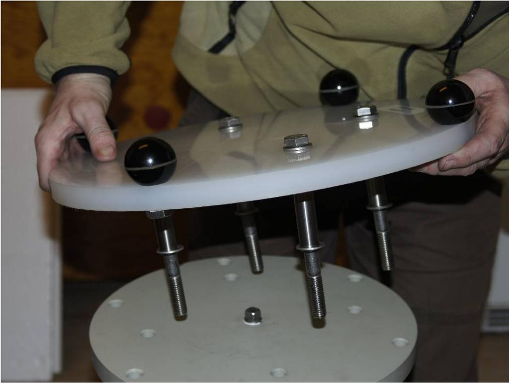
Fig. 6 Basic plate assembling to the column
