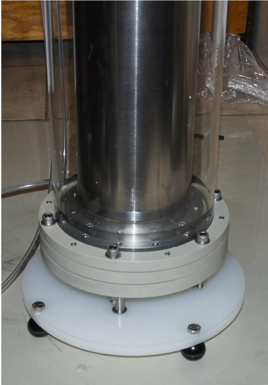
Fig. 9 Thermostating jacket – tube assembled
