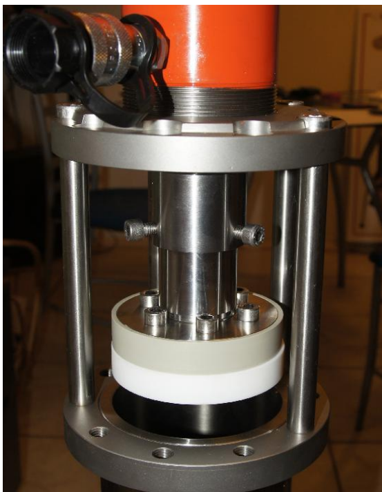
Fig. 7 Upper piston inserted on its position, connecting pieces fixed
