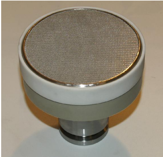
Fig. 5 Upper piston with seal rings
