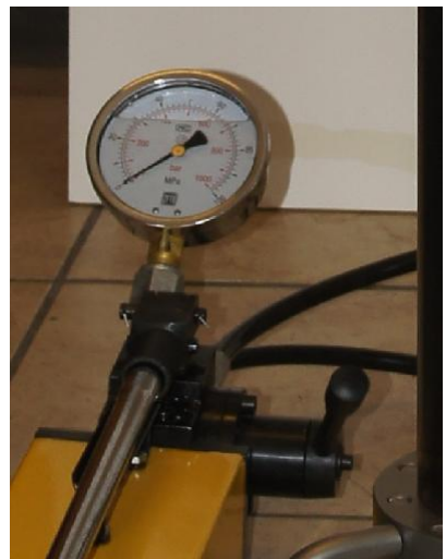
Fig. 8 Oil pump head with switching valve
