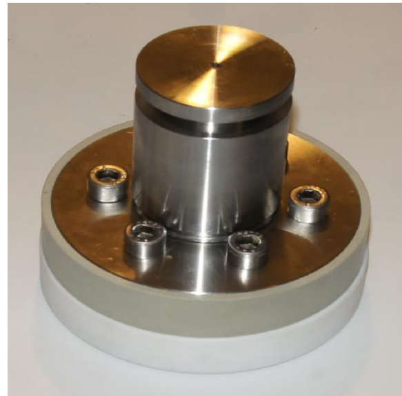
Fig. 6 Upper piston with support plate and connecting piece 1
